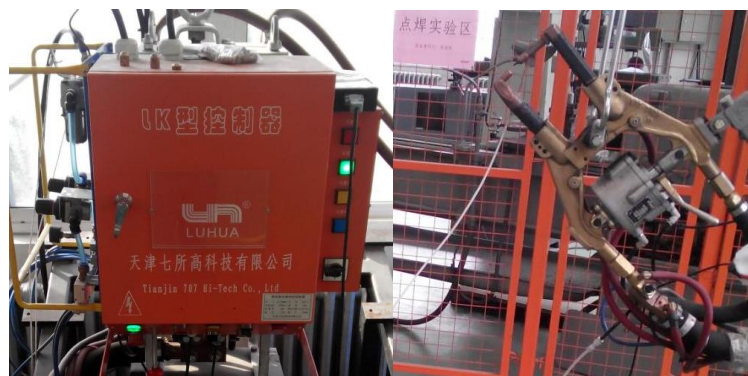
Figure 7. The control cabinet and welding tongs of the welding machine
