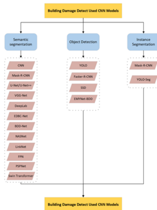
Figure. 6 The three main types of convolutional neural network models used for building damage detection tasks.
